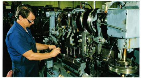
High quality parts featuring multiple bends and intricate cuts are processed at high speeds on this verti-slide forming press. It handles a full range of materials, from soft brass to molybdenum ribbon.
