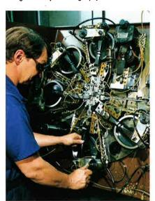
The complex workings of this high speed multislide press turn out between 300 and 600 multiple bend parts every minute. Starting materials cover a range from very thin wire gauges to one inch wide ribbon.
