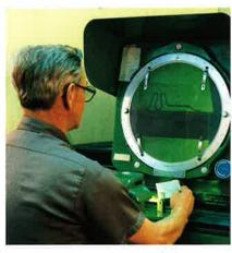
On the comparator, intricate formed wire parts are visually inspected at several times actual size to detect any dimensional variations that may be occurring because of tool wear or other small changes in the processing equipment.
