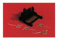
side-by-side in a plastic connector used in a wiring harness. The double looped end of the wire serves as a contact into which a ceramic printed circuit card is inserted. The wire is produced to a spring temper in this area to maintain uniform normal force throughout the life of the connection. The tail end of the wire is kept soft by segment annealing so it can be imbedded into the terminal body when the final connection is made. Quantities of parts like these are in the millions.
